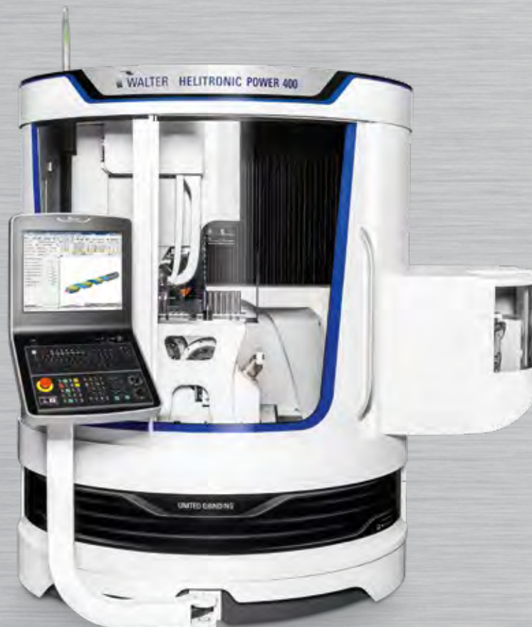
HELITRONIC POWER 400 with the options „Top loader“ and „Grinding wheel changer“ (right) – uncompromising in productivity and precision
