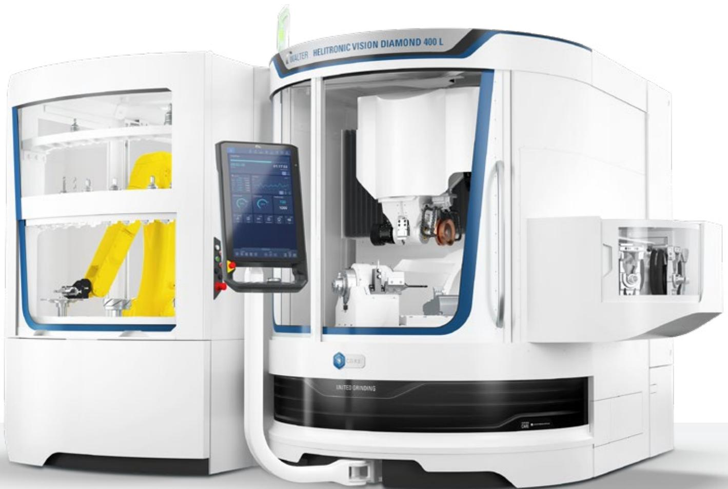
HELITRONIC VISION DIAMOND 400 L with the optional electrode/grinding wheel changer (right) and robot loader (left)
