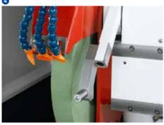
The most important component for complete machining is the wheelhead with integrated B-axis. It swivels automatically, and enables the use of up to four grinding wheels. This means that workpieces can be completely machined in the same clamping – with minimal auxiliary times combined with superior precision.
