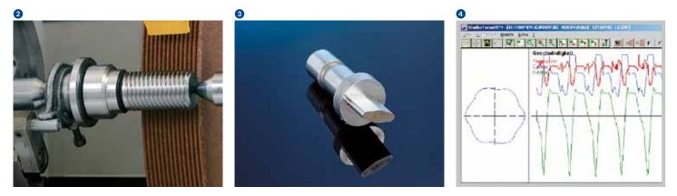
Complete machining also entails form and thread grinding operations to an ever increasing extent. These processes are made possible by the position and speed-controlled C-axis. The standard C-axis with measuring system on the drive motor is suitable for thread grinding. A direct measuring system is mounted on the workhead spindle (C-axis) to ensure the highest form accuracy). Acceleration and grinding forces are absorbed without difficulty through the high dynamic rigidity of the axis drives.
