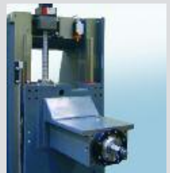
Grinding wheel head, drive and guideways and linear glass measuring scale for Y and Z axis (standard for a machine with easy Touch control)
