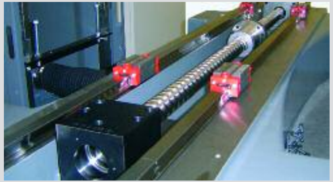
Precision guideways and high-quality, ground recirculating ballscrews in all axes
