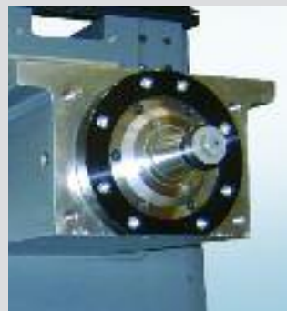
Cartridge type spindle with 4 precision ball bearing packs
