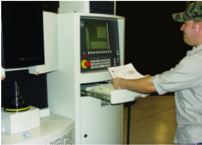
Corey inspects a step tool on the Walter Helicheck, with a repeatable accuracy of +/- 0.7 microns. West Ohio inspects the first and a random sampling of every 10th tool in a batch. "Tolerance to us, is a given," says Buck.
