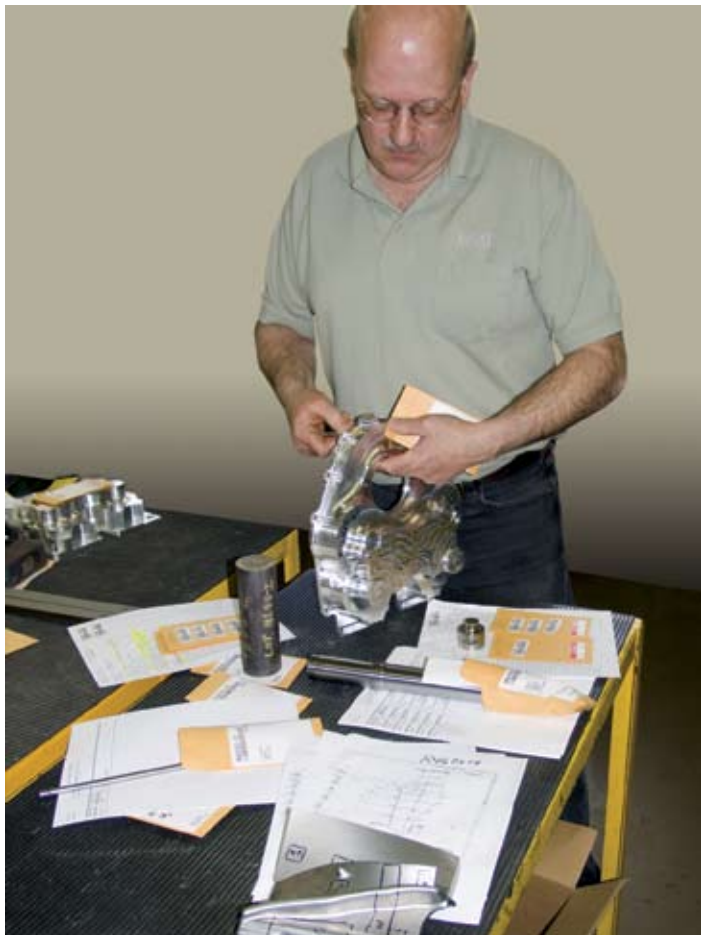
Machining Supervisor Richard Irwin looks over a wide variety of parts and material samples awaiting testing. These “raw” samples require machining to create a testable specimen (note the markings on the part in the foreground). As the paperwork suggests, Dirats Laboratories tracks each part throughout the process of machining and testing.
