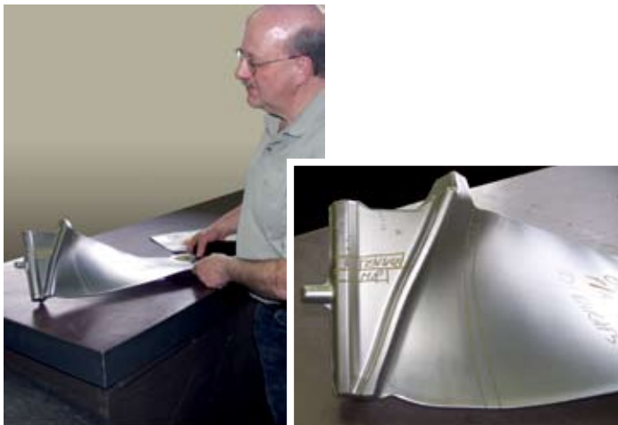
(pictured to the left) Turbine components are probably the most commonly tested item at Dirats Laboratories. Here Richard checks-in a just arrived forged blade. The markings indicate which sections need to be cut out and tested.
