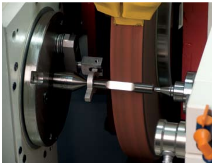
The Studer S31 has made out-of-round grinding an easy addition to Dirats Laboratories' capabilities, and the forms can be programmed off-line with StuderGrind
