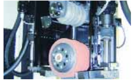
Overhead dressing system PEA-K for IPD and CD grinding methods designed for a grinding wheel width of up to 200 mm
