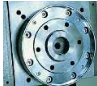
Cartridge type spindle with short taper for repeatable grinding wheel positioning
