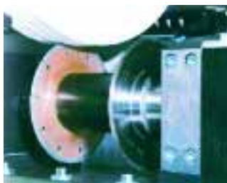
Fast initial profiling using a special roughing tool reduces the cost due to shorter cycles and less wear on precision tools
