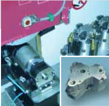
Housing for diesel injection pumps
