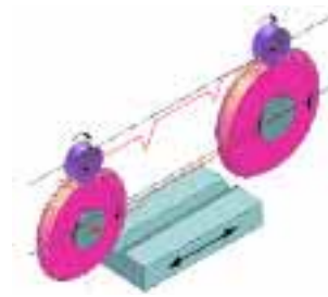
IPD-grinding, the in process dressing whilst grinding saves time and the possible grinding length is extended by the optimized grinding wheel topography
